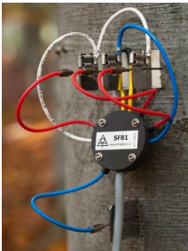
Sap Flow System produced by Environmental Measuring Systems, Ltd. (Brno, Czech Republic) installed on the tree trunk and the flows chart of measuring process. Sap flow values are calculated directly from the P/dT ratio (Nalevanková et al. 2020)
