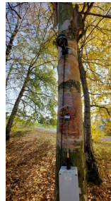
Sap Flow System produced by Environmental Measuring Systems, Ltd. (Brno, Czech Republic) installed on the tree trunk and the flows chart of measuring process. Sap flow values are calculated directly from the P/dT ratio (Nalevanková et al. 2020)
