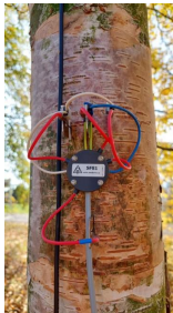
Sap Flow System produced by Environmental Measuring Systems, Ltd. (Brno, Czech Republic) installed on the tree trunk and the flows chart of measuring process. Sap flow values are calculated directly from the P/dT ratio (Nalevanková et al. 2020)
