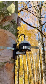
Sap Flow System produced by Environmental Measuring Systems, Ltd. (Brno, Czech Republic) installed on the tree trunk and the flows chart of measuring process. Sap flow values are calculated directly from the P/dT ratio (Nalevanková et al. 2020)
